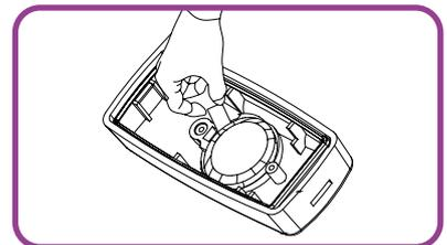
5. Refit the push button to the secured backing by offering up the button of the push button and gently pushing back together.
