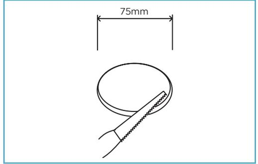
2) With a suitable position identified, carefully cut-out the recommended size based on the model you are installing.
