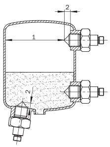
The apex should protrude into the container
