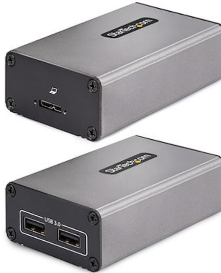
With this high-performance USB over Multimode Fiber Extender you can extend 5Gbps USB 3.2 Gen 1 signals over an OM3 LC to LC fiber cable with a range of up to 1150ft (350m).
