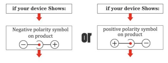
please choose the Negative Polarity side of the DC connector to Connect with the Adapter Please choose the Positive Polarity side of the DC Connector to connect with the Adapter
