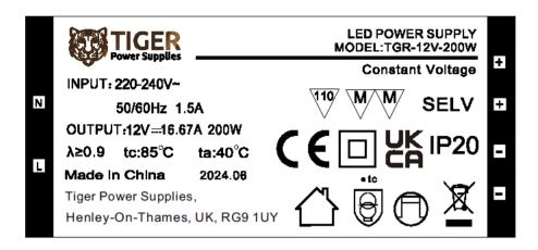
Please note the output is provided via 2 sets of terminal blocks. Each + and - set is capable of providing up to 10A (120W) max, with the total load of 16.67A (200W) only possible when using both + + and - output terminals
