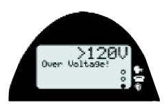
The PE830 automatically checks for high voltages and currents..
