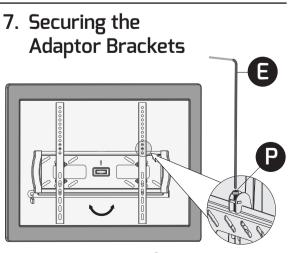
Tighten the top locking bolts () in the adaptor brackets, with the Allen key supplied, to secure the adaptor brackets to the wall plate.
