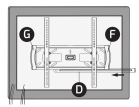
Slide the locking bar **①** through the guide in the base of the righthand End Cap **③** then through the guide in the two adaptor brackets and finally through the guide guide in the lefthand End Cap **⑤**.
