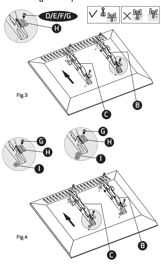
Select the correct size bolts to fit the VESA holes for your TV **①/③/⑥**. Attach the adaptor brackets to the back of the TV by lining up the VESA holes and using bolts **②/⑥/⑥**, the washers **①** and spacers **①** (if required) to fix the TV securely to the adaptor brackets.
