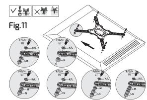
You can increase the spacing between the mounting plate and the back of the TV by using the spacers  $^{\odot}/^{\odot}$  see Fig.11.
