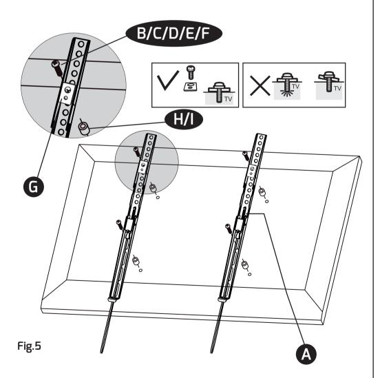
Select the correct size bolts to fit the VESA holes for your TV @/@/@/@. Attach the adaptor brackets to the back of the TV by lining up the VESA holes and using bolts <sup>⑤</sup>/**⑥**/**⑥**/**⑤**/**⑤**, the washers **⑥** and spacers **⑥**/**⑥** (if required) to fix the TV securely to the adaptor brackets.
