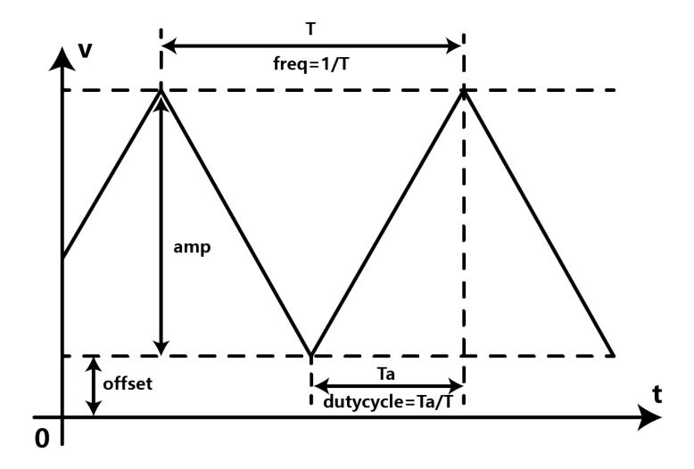
• Change the dutyCycle to 0 while the other parameters remain unchanged. That is "DAC.outputTriangle (5000,10,0,0)", which can generate a sawtooth wave of 5V in amplitude and 10Hz.
