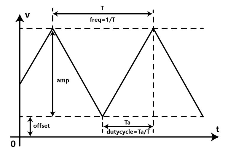
• Change the dutyCycle to 0 while the other parameters remain the same. That is "DAC.outputTriangle (5000,10,0,0)", which can generate a 10Hz sawtooth wave of 5V in amplitude.
