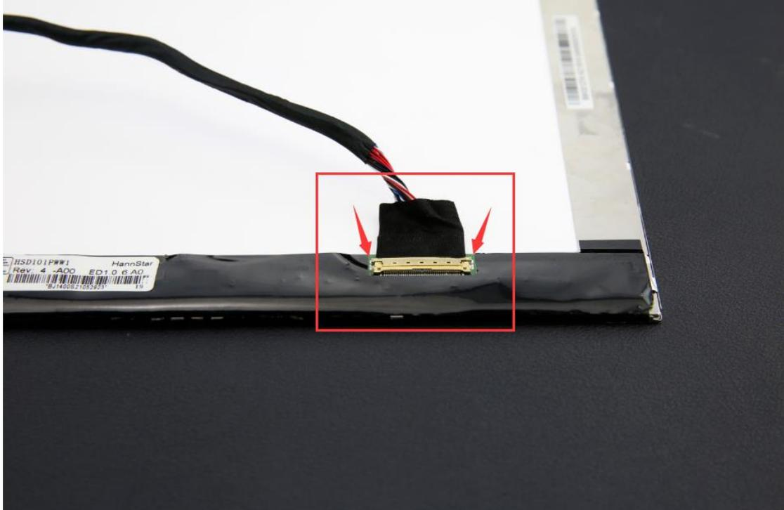
Step 2: Plug the LVDS cable on the driver board
