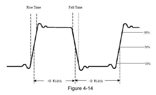
**Rise Time:** Time that the leading edge of the first pulse in the waveform takes to rise from 10% to 90% of its amplitude.
