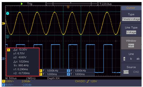
Figure 4-15 Time&Voltage Cursor Measurement
