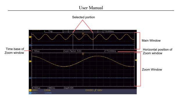
In normal mode, the **Horizontal Position** and **Horizontal Scale** rotary controls are used to adjust the horizontal position and time base of the Main window.
