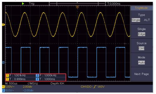
Figure 4-12 Automatic measurement
