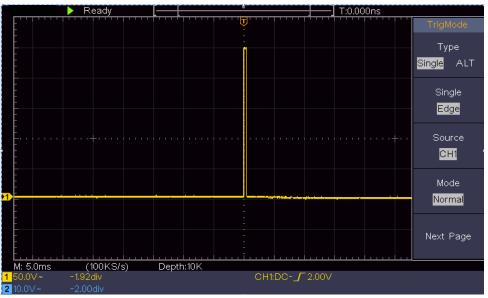
Figure 6-3 Capturing a Single Signal
