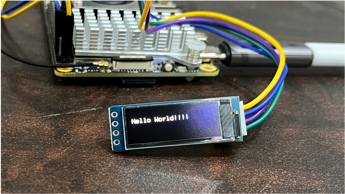
Fig. 5.22: Hello World!!!! on 128x32 OLED
