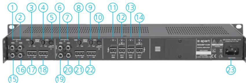
1. **Channel 4 overload led:** when this led lights up, you are overloading the input. Lower the input signal immediately to prevent distortion.
