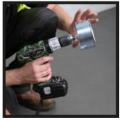
1. Attach the male spigot 2. Clamp the pipe to be into the drill chuck.
