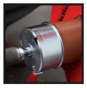
3. Engage the drill and rotate the tool, keeping it parallel to the pipe.
