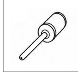
3. **Adaptor (12)** is used for rubber dinghies, inflatable small swimming pools and air beds.
