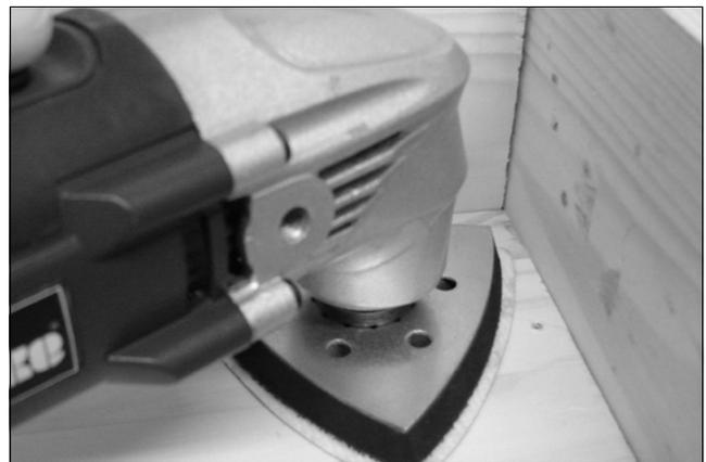
**NOTE:** The sanding pad must be kept flat on the workpiece. Take care not to tilt the base and use the edge of the pad. This will damage the sanding sheet and pad, making it harder to grip the sanding sheet.
