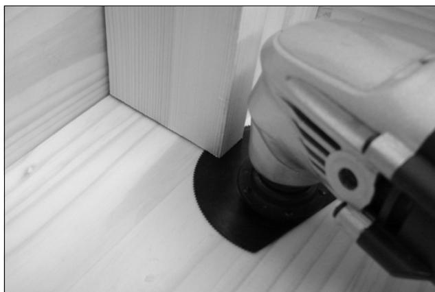
**NOTE:** If using the saw attachments for plunge cuts, only use the saw on soft materials such as softwood and plaster boards. Always check that there are no nails or screws in the workpiece before cutting.
