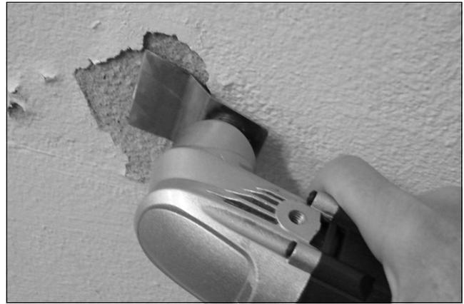
**NOTE:** The scraping blade is designed for scraping soft materials from flat surfaces. Ensure you get the correct angle and only apply light pressure to avoid cutting the surface.
