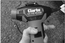
For continuous inflation you can push the switch lock upwards to lock while the On/Off trigger is depressed. In this way, inflation continues without pressing any button. To stop, simply squeeze the trigger to release the locking switch.
