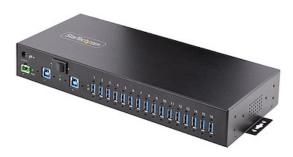
The 16-Port Industrial USB 5Gbps Hub with Power Adapter features 16 downstream USB-A ports. The rugged all-metal construction is suitable for use in industrial rackmount applications. Level-4 Electrostatic Discharge (ESD) protection safeguards against 15kV Air / 8kV Contact discharges. The hub features a 2-port host switch, enabling users to switch between two host devices.
