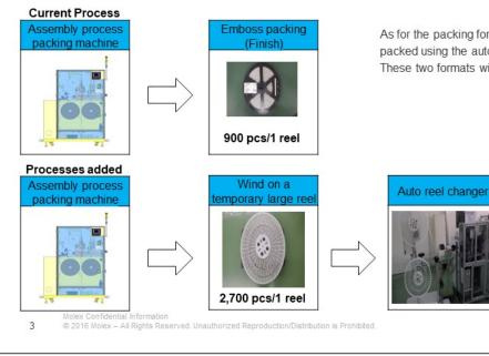
As for the packing form, the embossed packing form packed using the auto reel changer will be added. These two formats will exist in the future.
