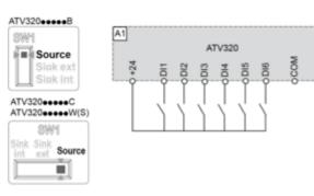
Switch SW1 set to "Source" position and use of an external power supply for the DIs.
