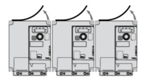
Mounting Type C: Individual, Ventilation Cover Removed
