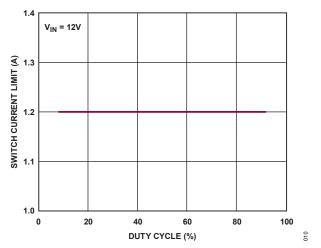
Figure 12. Switch Current-Limit vs. Duty Cycle
