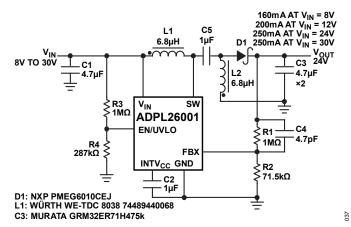
Figure 38. 8V to 30V, 24V SEPIC Converter
