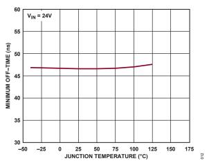
Figure 14. Switch Minimum Off-Time vs. Temperature
