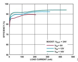
Figure 33. Efficiency vs. Load Current (Figure 32 Circuit)
