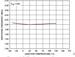
Figure 9. Switching Frequency vs. Temperature
