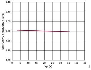
Figure 10. Switching Frequency vs. V<sub>IN</sub>
