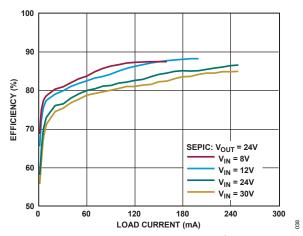
Figure 39. Efficiency vs. Load Current (Figure 38 Circuit)
