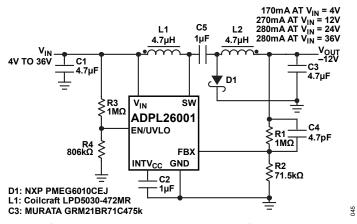
Figure 46. 4V to 36V Input, -12V Inverting Converter
