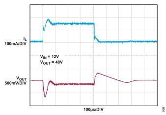
Figure 22. V<sub>OUT</sub> Transient-Response: Load Current Transients from 5mA to 135mA to 5mA (Figure 30 Circuit)
