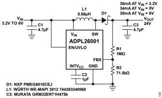
Figure 36. 3.2V to 6V, 24V Boost Converter
