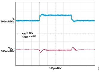
Figure 21. V<sub>OUT</sub> Transient-Response: Load Current Transients from 67.5mA to 135mA to 67.5mA (Figure 30 Circuit)
