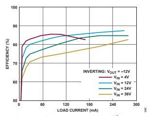
Figure 47. Efficiency vs. Load Current (Figure 46
