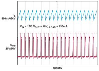
Figure 18. Switching Waveforms (Figure 30 Circuit in CCM)
