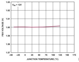
Figure 6. FBX Positive Regulation Voltage vs. Temperature
