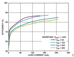
Figure 45. Efficiency vs. Load Current (Figure 44 Circuit)
