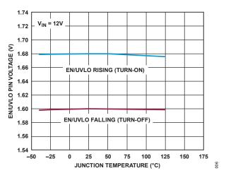
Figure 8. EN/UVLO Pin Thresholds vs. Temperature
