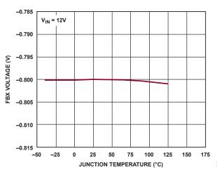
Figure 7. FBX Negative Regulation Voltage vs. Temperature
