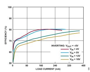
Figure 49. Efficiency vs. Load Current (Figure 48 Circuit)
