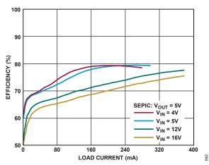
Figure 43. Efficiency vs. Load Current (Figure 42 Circuit)
