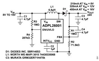
Figure 32. 8V to 16V Input, 24V Boost Converter
