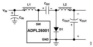
Figure 29. A Simplified Inverting Converter
