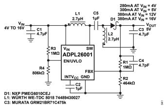
Figure 42. 4V to 16V Input, 5V SEPIC Converter
