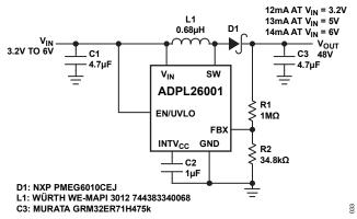
Figure 34. 3.2V to 6V Input, 48V Boost Converter
