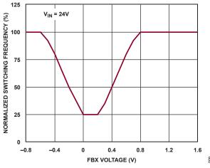
Figure 11. Normalized Switching Frequency vs. FBX Voltage
