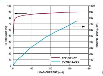
Figure 2. Efficiency and Power Loss vs. Load Current (Figure 30 Circuit)
