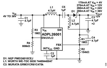
Figure 40. 4V to 36V, 12V SEPIC Converter
