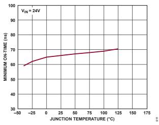
Figure 13. Switch Minimum On-Time vs. Temperature
