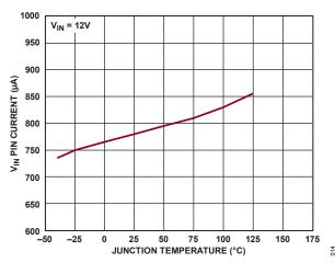
Figure 16. V<sub>IN</sub> Pin Current (Active Mode, Not Switching) vs. Temperature
