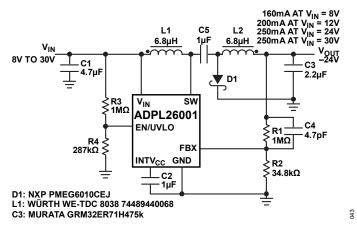
Figure 44. 8V to 30V, -24V Inverting Converter
