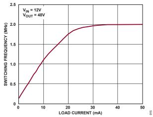
Figure 17. Burst Frequency vs. Load Current (Figure 30 Circuit)
