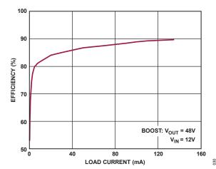
Figure 31. Efficiency vs. Load Current (Figure 30 Circuit)
