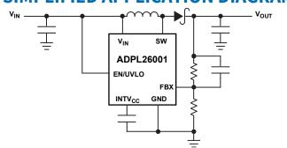
Figure 1. Simplified Boost Converter
