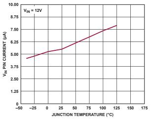
Figure 15.  $V_{IN}$  Pin Current (Sleep Mode, Not Switching) vs. Temperature
