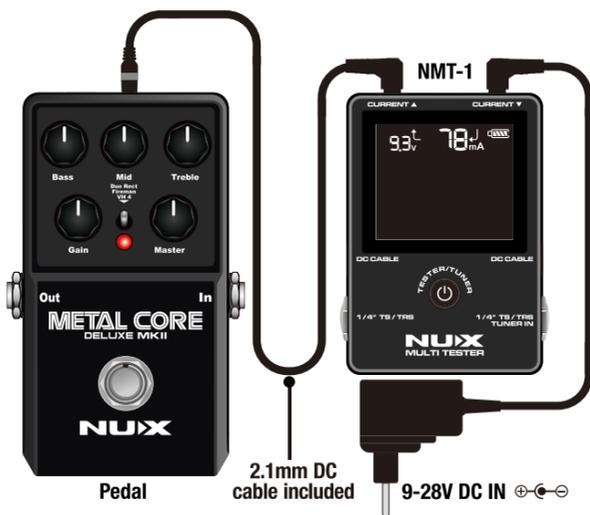
\*You can also plug the short DC cable into the daisy-chain cable from NMT-1 to measure the total current draw of your pedal board effects.
