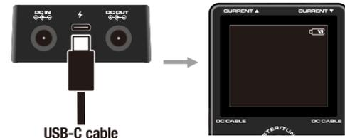
NMT-1 takes power from Li-on battery and can be charged through the USB-C port. You can use the included USB-C cable to connect your power supply.
