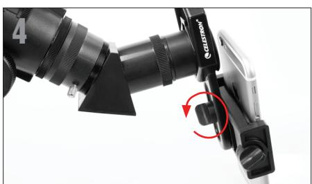
Loosen the knob on the bottom of the adapter that secures the phone clamp to the eyepiece clamp. Slide the phone clamp up and down and rotate it left and right until your camera is looking down through the eyepiece of the telescope. Tighten the knob on the bottom of the adapter to secure it in place.
