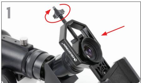
Open the eyepiece clamp and place it around the body of the eyepiece. Tighten the clamp until it's secure.
