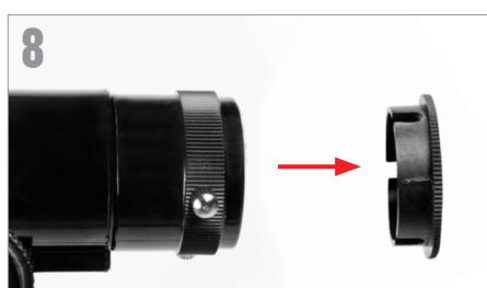
Remove the cap from the focuser end of the telescope tube and make sure the two thumbscrews do not protrude into the opening.
