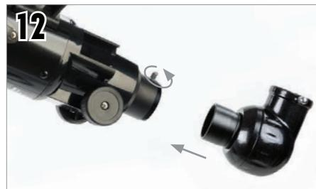
Locate the diagonal and remove the plastic covers. Insert the barrel of the diagonal into the focuser and secure in place by tightening the set screws.
