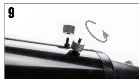
Remove the knurled nuts on the threaded posts at the focuser end of the telescope tube.
