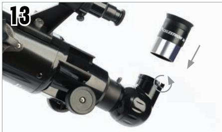
Insert the barrel of the 20mm eyepiece into the diagonal and tighten the set screw, being careful not to overtighten.
