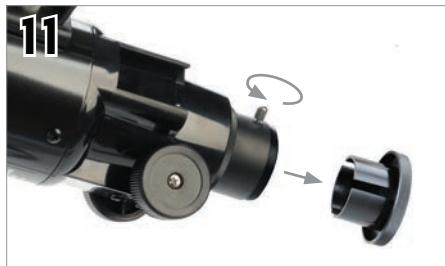
Loosen the screws on the focuser so they do not obstruct the inner diameter of the focuser. Remove the plastic cap covering the end of the focuser.
