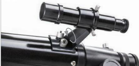
Locate the finderscope and remove plastic caps on front and back of lens. Orient the finderscope so that the longer lens is facing towards the front of the tube as shown here. Place finderscope over the posts on the tube and replace knurled nuts to secure.
