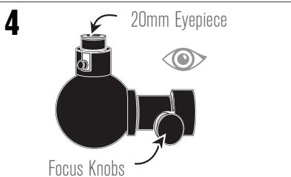
Look through the telescope's 20mm eyepiece. Gently turn the focus knobs to adjust the sharpness of the image.
