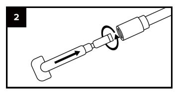
Insert tip and rotate to engage the male end into the handle recess.
