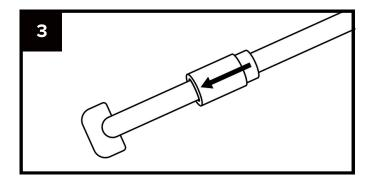
Release the collar once the tip is fully inserted.
