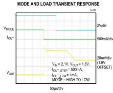
$(MAX38911, V_{IN} = 2.1V, V_{OUT} = 1.8V, T_{A} = +25^{\circ}C, C_{IN} = 4.7 \mu F, C_{OUT} = 4.7 \mu F, C_{BYP} = 10 nF, unless otherwise noted.)$
