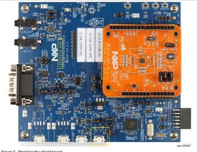
Figure 2. Stacking the shield board
