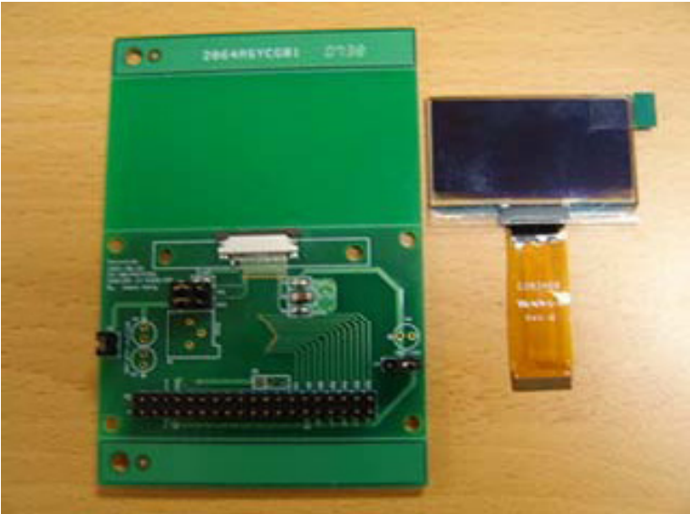
Figure 5 EVK PCB and DD-12864YO-3A Module
