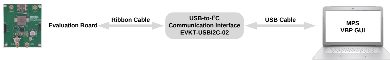
Figure 1: EVKT-MPQ4242B Evaluation Kit Set-Up
