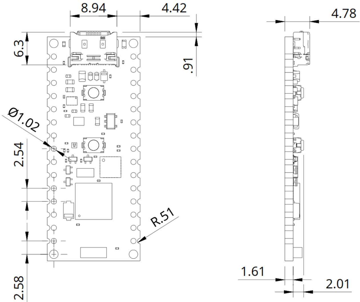
The Nano Matter was designed to be usable as a surface-mount module and presents a dual inline package (DIP) format with the Nano-styled header connectors on a 2.54 mm pitch grid with 1 mm holes.
