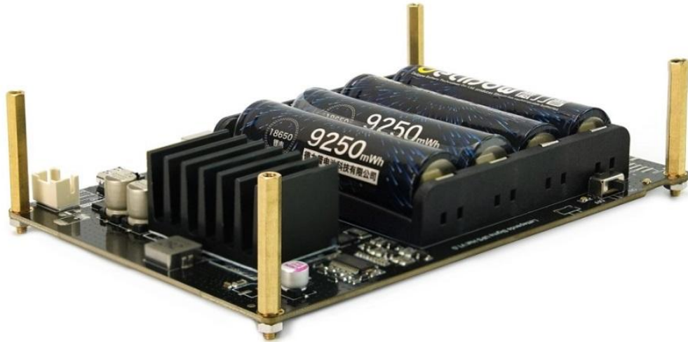
Figure: Install the 18650 lithium battery into the the LattePanda Sigma development board
