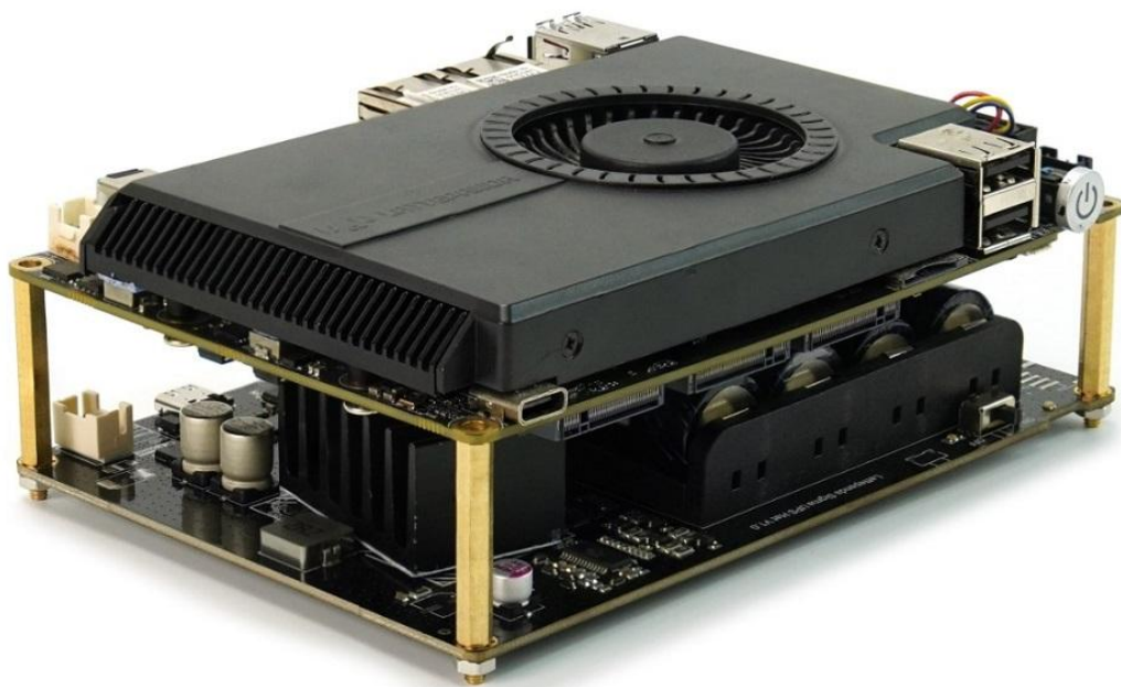
Figure: Mounting the UPS to the LattePanda Sigma Single Board Computer
