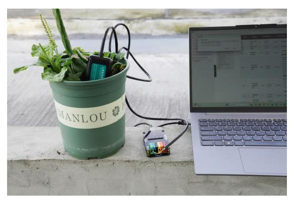
Figure: Wiring RS485 soil sensor and RainbowLink Converter to Detect Soil Moisture
