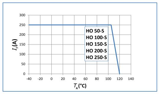
Important notice: whatever the usage and/or application, the transducer primary bar temperature shall not go above the maximum rating of 120 °C as stated in page 3 of this datasheet.
