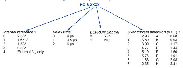
$\begin{array}{c} \textbf{Standard products:} \ \ \text{HO 50-S-0100; HO 100-S-0100; HO 100-S-3110; HO 150-S-0100; HO 200-S-0100; HO 200-S-0100; HO 250-S-0100; HO 250-S-010D \end{array}$
