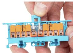
Remove the jumper from open clamping units.
