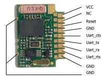
= Power Supply = UNUSED = Full Hardware Reset (active low) = Ground Cts = « Clear to send » Control Signal In bx = « Data to transmit » Data Out rx = « Received data » Data In rts = « Request to send » Control Signal Out = Ground = Ground
