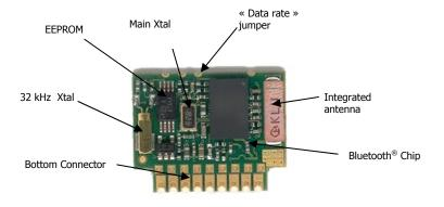
**Pin-out** All connections are located on the A<sup>*RF32*</sup> bottom connector:
