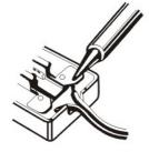
Apply rosin-based solder to the part and melt it with the soldering iron.
