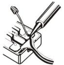
Wait for the solder to cool and harden before moving the soldered part.
