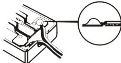
**Note:** Lightly dampen the sponge with water before use. Before soldering, clean the tip on the sponge and then tin the tip with fresh solder. Do not use the sponge dry.
