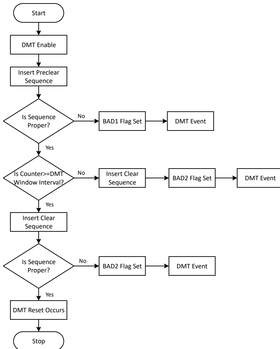
Figure 21-2. Flowchart for Clearing the DMT
