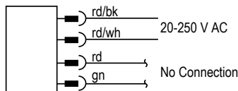
4-pin 1/2 in-20UNF (1/2-in Dual Key) quick disconnect emitters
