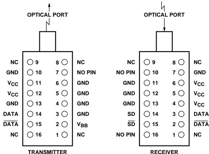
Figure 3. Pinout drawing.
