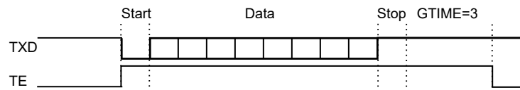
Figure 30-15. Example of TE Drive with Guard Time
