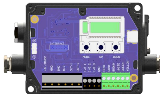
Blue electronic board for LTfast, P3, P7, and xM
