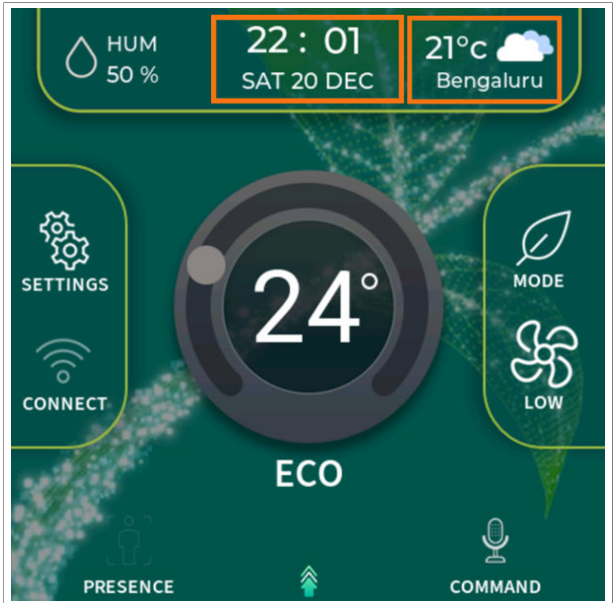
Figure 22 Weather, temperature and time update through HTTP server
