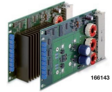
The ADS\_E is a powerful pulse-width modulated (PWM) Servoamplifier for controlling permanent magnet activated DC motors of 10 – 500 watts. Available in Eurocard format as Standard and Power Version.
