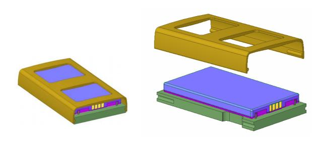
Once again mechanical fixation of the pack towards x and y direction is give by the L-shape recesses in the pack itself and fitting L-shaped noses in the customer device. The z-axis is fixed by cover – which in this case is sided onto the base plate. An additional sponge within the cover will compensate for tolerances.
