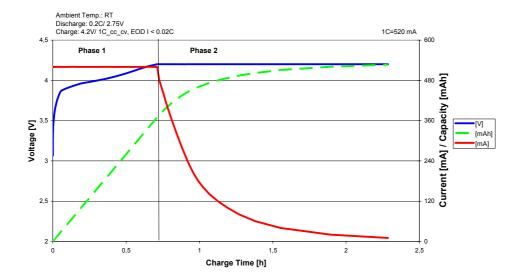
Above figure illustrates the different phases during a rapid charge cycle. The battery in this example is a VARTA EasyPack 550, discharged down to 3.0V. So the battery is empty.
