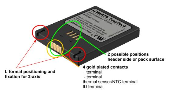
For mechanical integration, VARTA EasyPack incorporates two L shaped positioning recesses, which fix the pack mechanically in your device. 3D CAD models, available through VARTA Microbattery local sales offices, allow the simple design of fitting counterparts into your housing. Gold plated contacts (2.5mm pitch) give reliable electrical interconnection. Fitting contact blocks for your own PCB are available from multiple sources.
