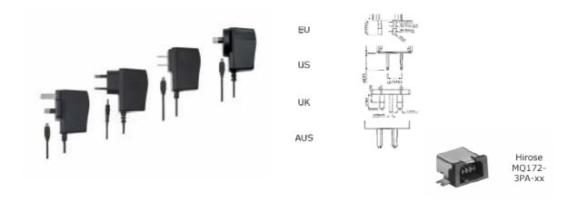
At this point in time RRC Power Solutions offers an EasyPack compliant wall plug charger (part number RRC EPC06WC) . The charger is a universal solution with a fixed cc/cv of 750mA/4.2V. Below table indicates the typical charge time for the different EasyPack sizes.
