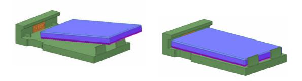
An additional device cover closes the battery casing.
