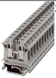
Universal terminal block with screw connection, cross section: 0.5- 10 mm², AWG: 20- 6, width: 10.2 mm
