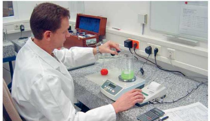
The different components of a mixture can be weighed in with the formula function. The total weight of all the components can be called up for control purposes. Documentation of the mixture is possible with the standard printers KERN YKB-01.
